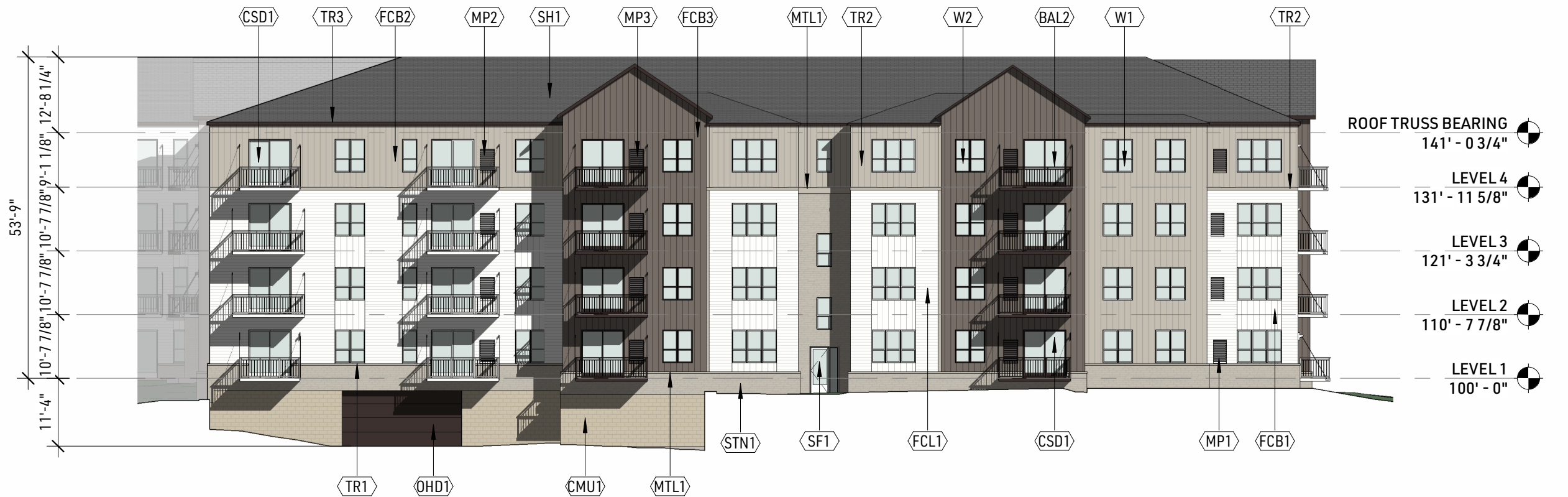
1 ELEVATION - WEST - SOUTH PORTION 1" = 20'-0"
