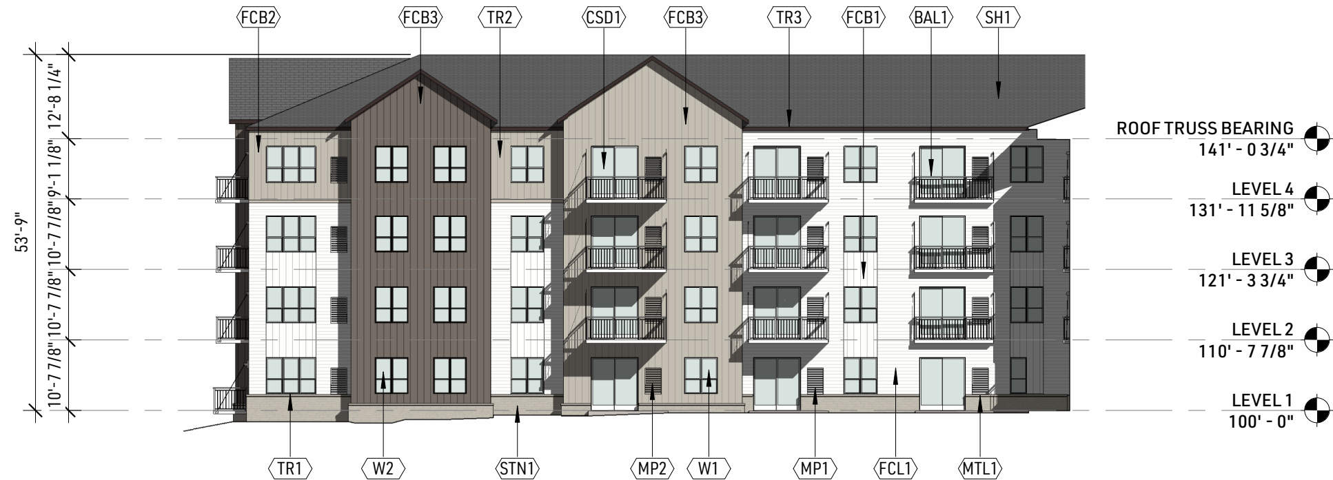
2 ELEVATION - WEST INTERIOR COURTYARD 1" = 20'-0"
