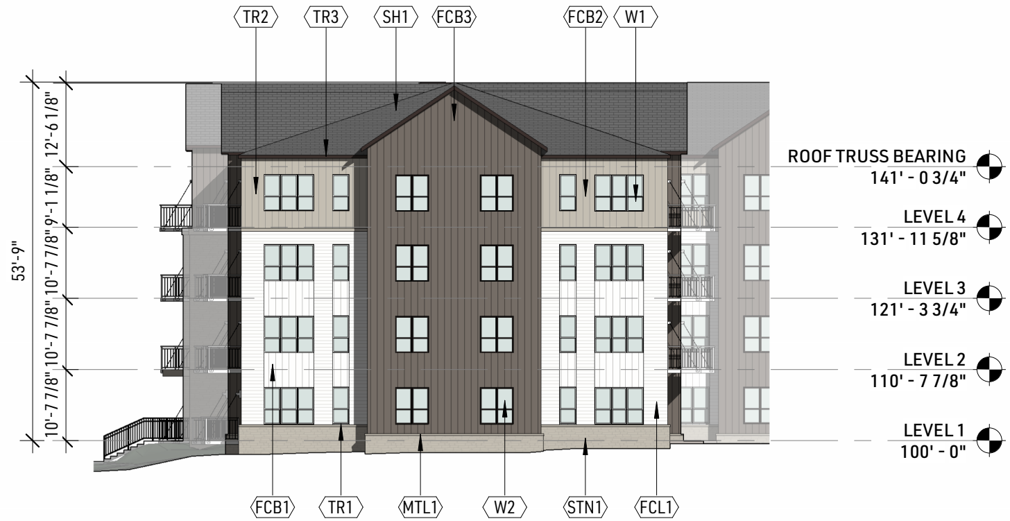
2 ELEVATION - NORTH - WING 1" = 20'-0"
