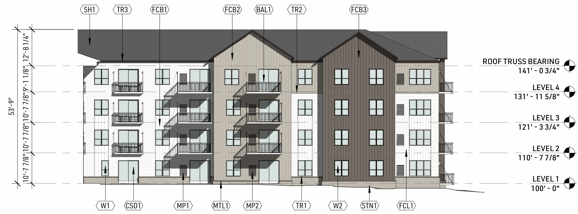
1 ELEVATION - EAST INTERIOR COURTYARD 1" = 20'-0"
